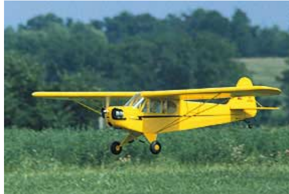
Figure 2. Sig Manufacturing quarter scale Piper J-3 Cub kit, basis of primary air vehicle
